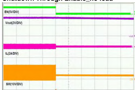
Shutdown Through Enable_no load
