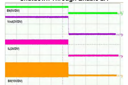
Shutdown Through Enable 2A
