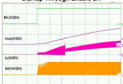
Startup Through Enable 2A
